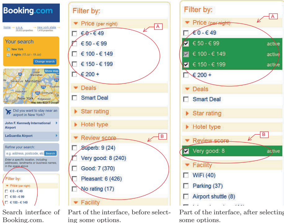
Figure 2.2: A complex, faceted search form in which the typical behavior of a checkbox is altered. Normally, from a group of checkboxes, you can select any number of options, as is the case in group A. However, in group B, as soon as one option is selected, the other options disappear.
